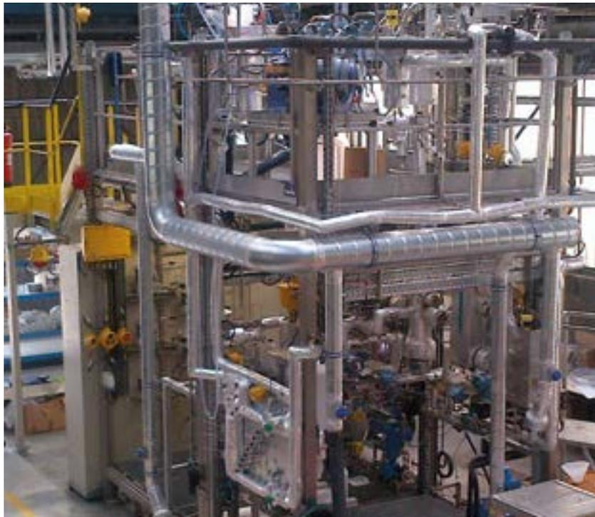
IFP Energies Nouvelles (IFPEN) owns a dedicated pilot testing facility in its premises of Solaize. Dedicated tests can be done upon client's request with a reconstituted gas to confirm the performance of the process for any new application (cf. Figure 3).
