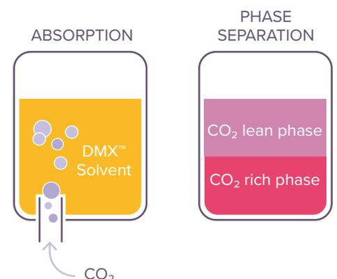
↑ Figure 1: The demixing principle
