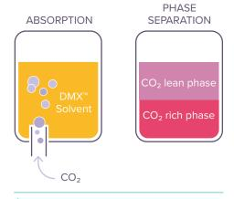
↑ Figure 1: The demixing principle
